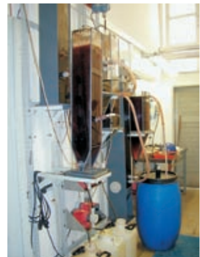
The pilot model of biological waste water treatment
