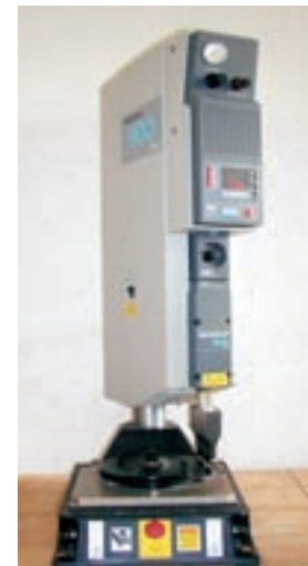
Ultrasonic welder of membranes
